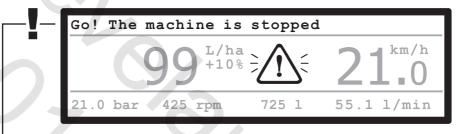
Disable spraying command! Go! The machine is stopped Start pump! No flowrate Go slow! High pressure Go fast! Insufficient pressure Go fast! Insufficent flowrate Go fast! High flowrate Reduce rotation speed! Increase rotation speed! Stop immediately! Pump fault Flowmeter out of range SD card not found! SD card write protected! SD card full! SETUP.BIN: File not found!
